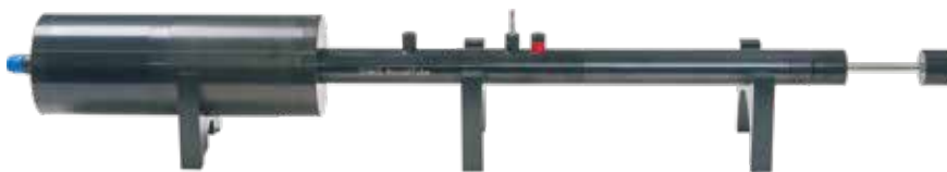
//Photo: Impedance tube for acoustical measurements
